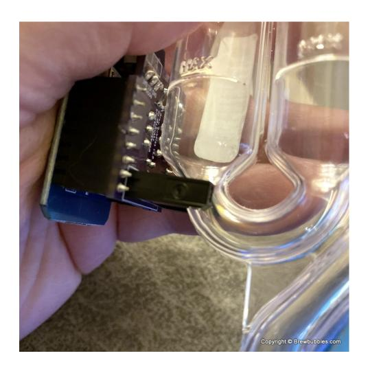
The airlock is then passed through the hole in the bracket and into the carboy stopper. The hole may need to be adjusted larger or drilled out depending on the size of your airlock. If it is too loose around the airlock, a drill stop or even tape may be used on the tube under the bracket to hold it in place.
