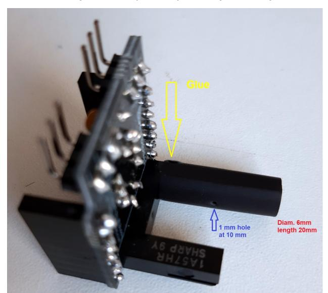
And here, wd16261 uses a piece of shrink-tubing with a dot of glue to hold his pinhole camera in place:
