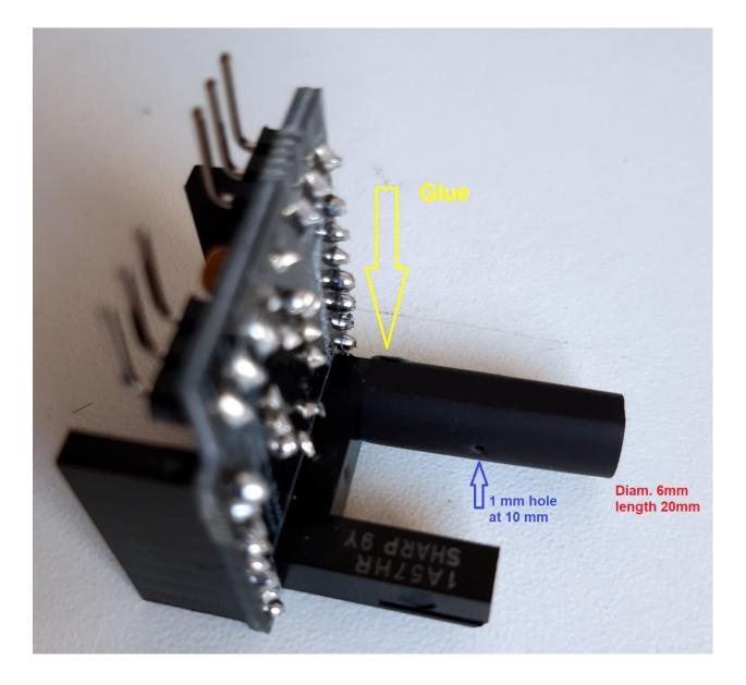
Both of these form collimators that restrict the amount of light entering the sensor. Both seem to be very effective and likely simpler than messing with light filters.
